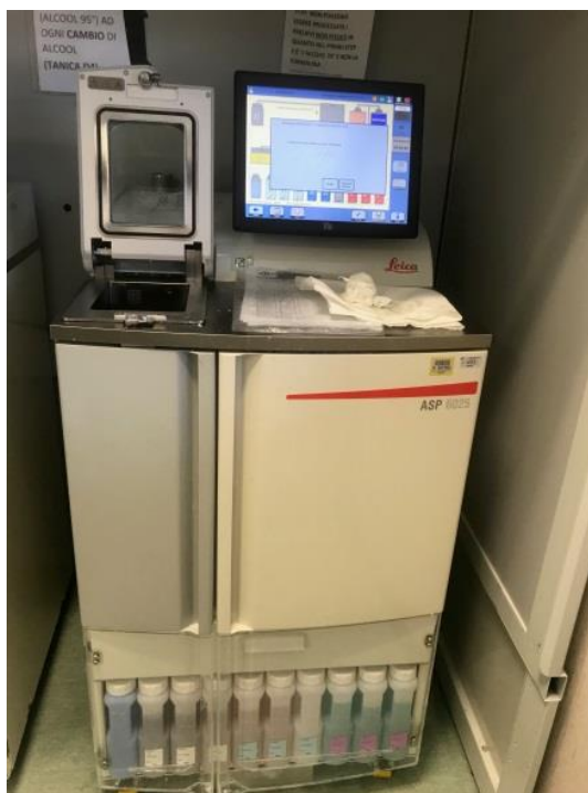
Figura 10. ASP6025 Automated Vacuum Tissue Processor
